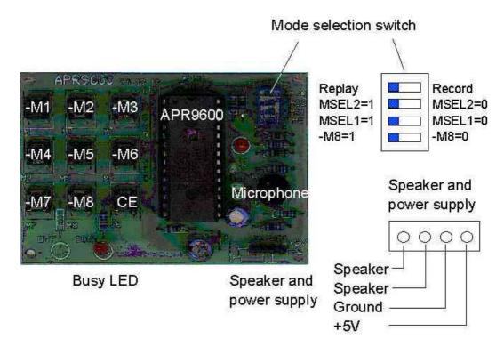
Figure 3 APR9600 module with connector details (to record in parallel mode, the switch setting should be same as displayed above. To record, the top switch should be on the right-hand side. To replay, the top switch should be on the left)
