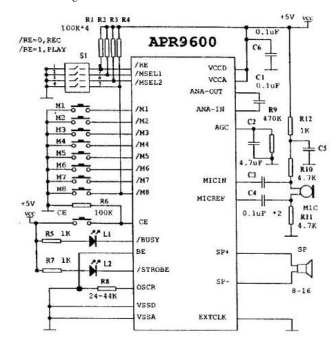
Figure 2 Typical connections of the APR9600
