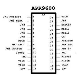
Figure 1 Pin-out of APR9600
